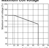
Ambient temperature (°C) Note: The maximum coil voltage is the maximum voltage that can be applied to the relay coil
