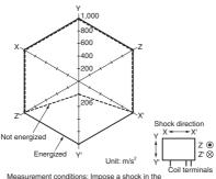
Measurement conditions: Impose a shock in the  $\pm X$ ,  $\pm Y$ , and  $\pm Z$  directions three times each with the Relay energized to check the shock values that cause the Relay to malfunction.
